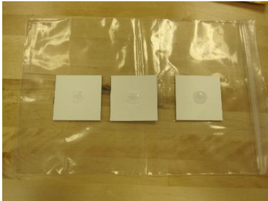
Photo No. 1 ASTM D1308 Testing in Progress
